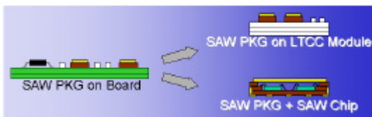
Figure 4: Market trend of ceramic SMD packages for SAW filters
